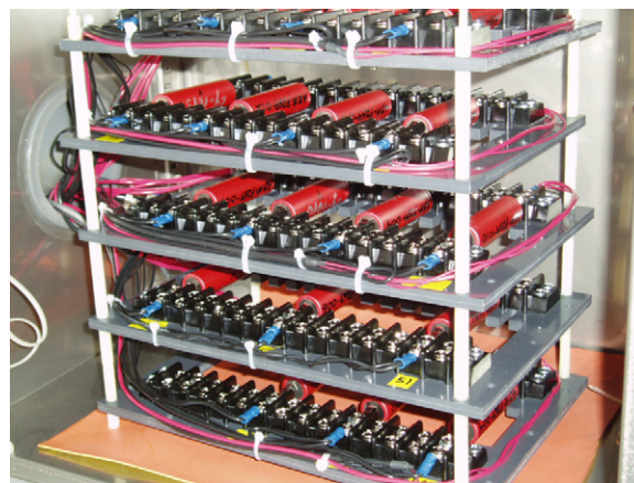
Fig. 1. Photograph of selected 18650 Sanyo Y cells on test at the INL, as placed within an environmental chamber.
